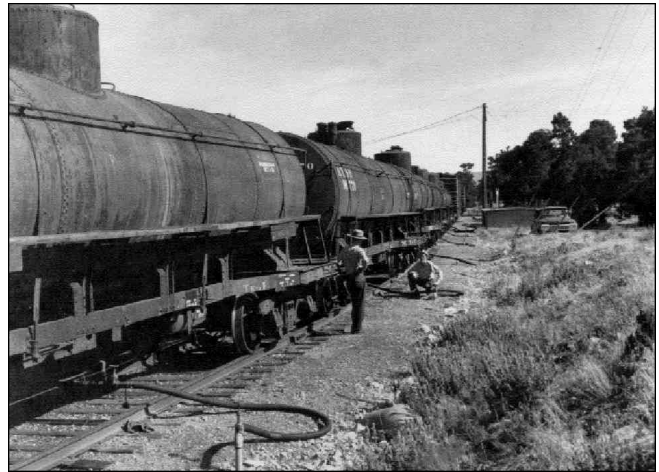
Figure 17. Twenty 10,000-gallon tankers deliver water from the Chinle Valley to South Rim storage tanks, 1961. The Santa Fe supplied water in this manner from 1901 until the late 1960s—daily until 1932 and as needed thereafter. GRCA 3605.
